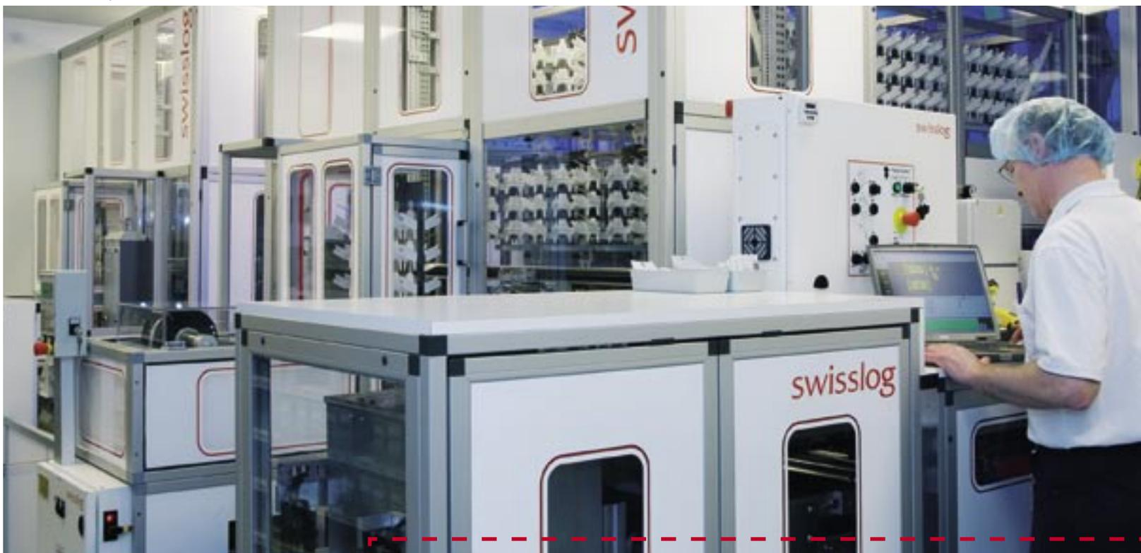
▲ The equipment at Århus University Hospital, Skejby consists of two dose dispensing robots placed in a clean area at the pharmacy. The robot is for the moment operated by two technicians and a pharmaconomist - in this picture JØRGEN HANSEN is supervising the operation.
